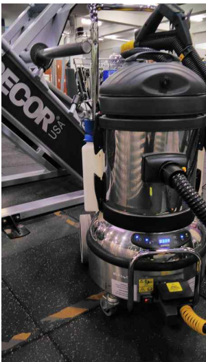
Steam cleaning(180°C) for gym mat. Work in progress: https://youtu.be/s_VM3AEOexE
